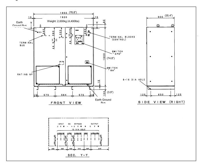
Figure 5 - 300kVA UPS Exterior dimensions (front & right side).
